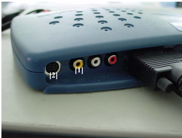
Figure 17: Output sockets of Marvel G400-TV detail
