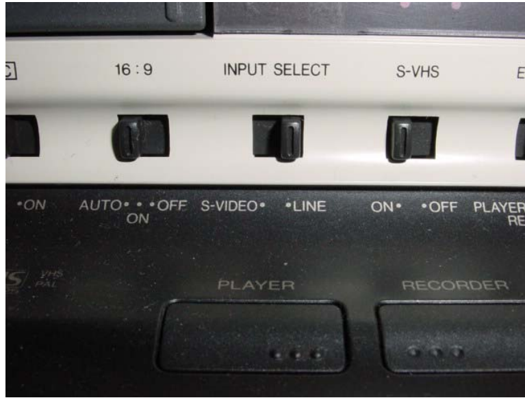
Figure 12: INPUT SELECT switch detail
