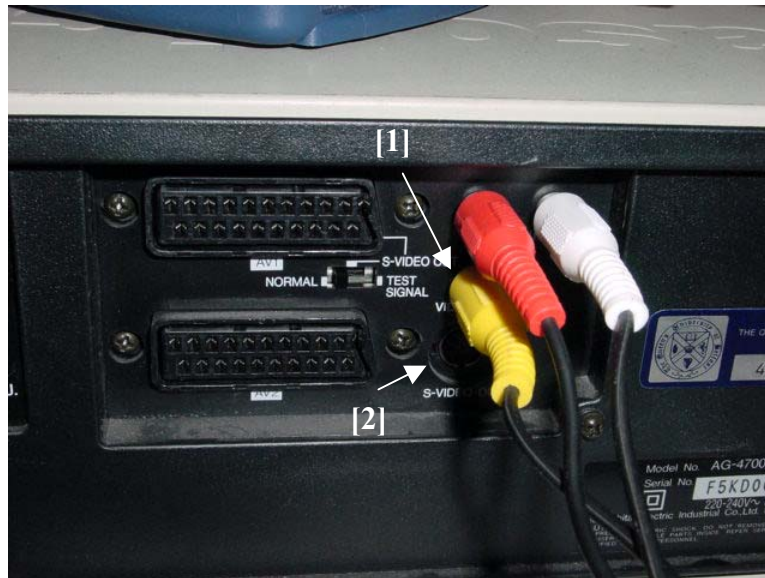
Figure 15: VCR video output detail
