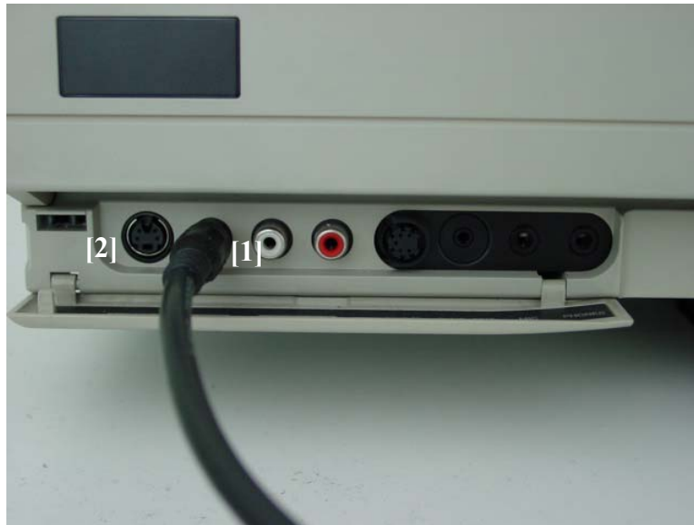
Figure 11: VCR video input AV3 detail
