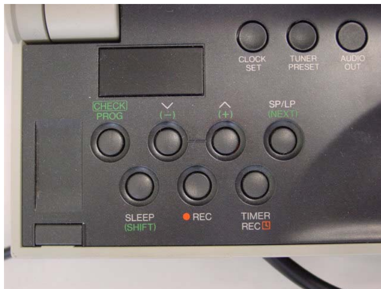
Figure 13: VCR control panel detail
