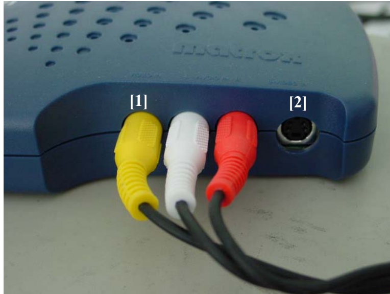
Figure 16: Input sockets of Marvel G400-TV detail
